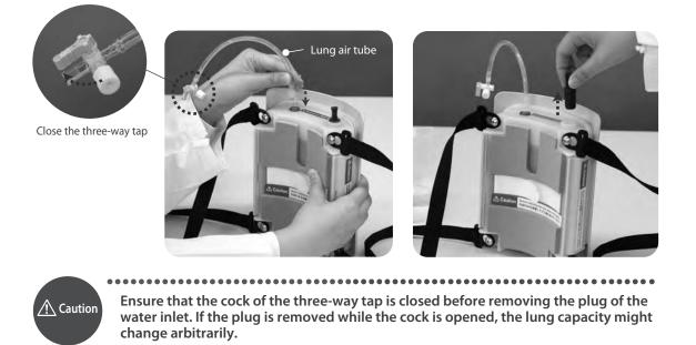
2. When you extract the air from lung, connect the empty syringe to the three-way tap and lock it by turning clockwise. Pull the plunger while setting the three-way tap in the open position. When you air the lung, fill the syringe with air and connect it to the three way tap. Lock it by turning clockwise. Put the plunger while setting the three-way tap in the open position. After adjusting the lung size, close the cock of the three-way tap and remove the syringe from the tube.
