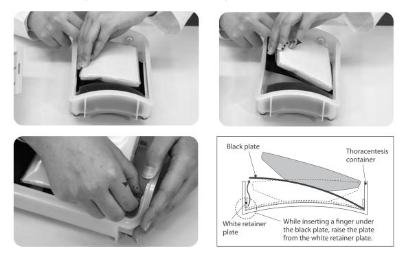
2. Replace with the new simulated lung, and then connect the tube from the lung to the lung air adjustment pipe located on the top of the thoracentesis container. Then insert the edge of the black plate under the white retainer plate. First, put one of the edges of the black plate under the retainer plate and then push the other side of the black plate under the retainer plate on the other side to install the simulated lung.
