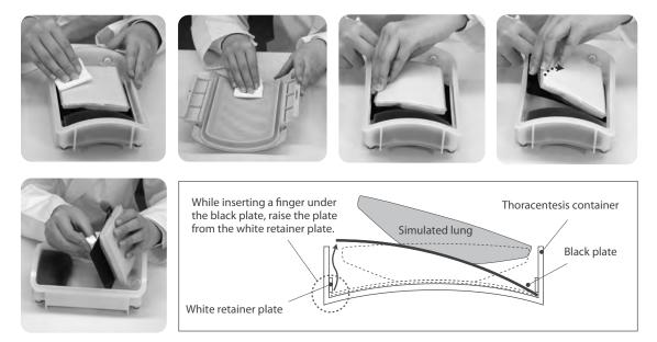
6. After the moisture is wiped off completely, reset the simulated. Insert the edge of the black plate under the white retainer plate. First, put one of the edge of the black plate under the retainer plate and then push the other side of the black plate under another retainer plate.
