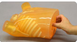
Insert the diaphgram block until the bottom of the block and the edge of the phantom body come to the same plane without a step.
