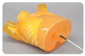
6. Please take opposite step described above in detaching the lung field. In case the phantom is demounted in the upper side, it becomes easier to detach by pushing downward the projection at the tip of heart from the hole in the neck.
