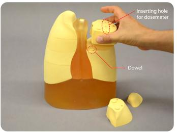
3. Laminate the lung field by putting the uneven parts (circle) together.
