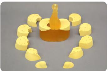
2. Then assemble the lung field units. Lung field consists of 6 laminated parts both in left and right part. Dosemeter can be put in the inserting hole of laminated parts.
