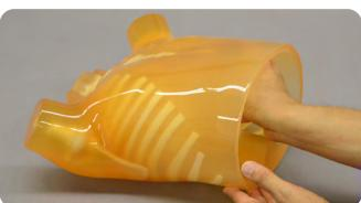
2. Insert heart deeply until its top reaches to the neck of the phantom. Adjust its angle so that the projection at the tip of heart fit the hole in the neck. Peeping through the neck hole to check the angle while advancing the insert helps smooth insertion.
