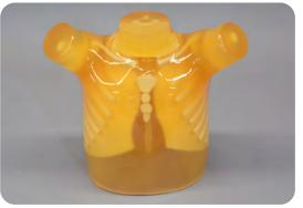
5. Both for lung vesculature and lung density inserts lon chamber can be inserted to the opening at the the bottom of diaphgram.
