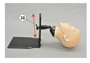
3. The phantom is ready. Adjust the height of the neck as needed, by loosen the fixture and slide it through the slit. Tighten the fixture again at the
