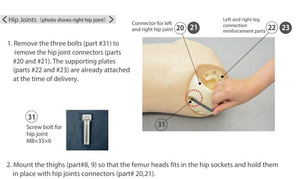
Each hip joint connector is fixed to the trunk with three screws. Start from the screw in the center and move to the sides. Hold the thigh upright when you fix the screw at the rear end. Be careful not to confuse parts for left and for right.
