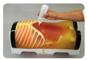
2. Spread ultrasound gel over the phantom body.
