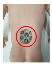
2. Connect the yellow outlet tube to the yellow connector labelled '1. Urine outlet' (identified by the two-tone yellow ring). Place the open end of the tube into an empty fluid container to collect excess fluid
